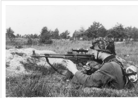
A soldier demonstrates the transitional MP 43/1 variant, used to determine the suitability of the rifle for sniping purposes, October 1943. The rifle is fitted with a ZF 4 telescopic sight.
