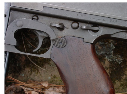
Fire Controls M1 Thompson Front lever is selector switch set for full auto.
